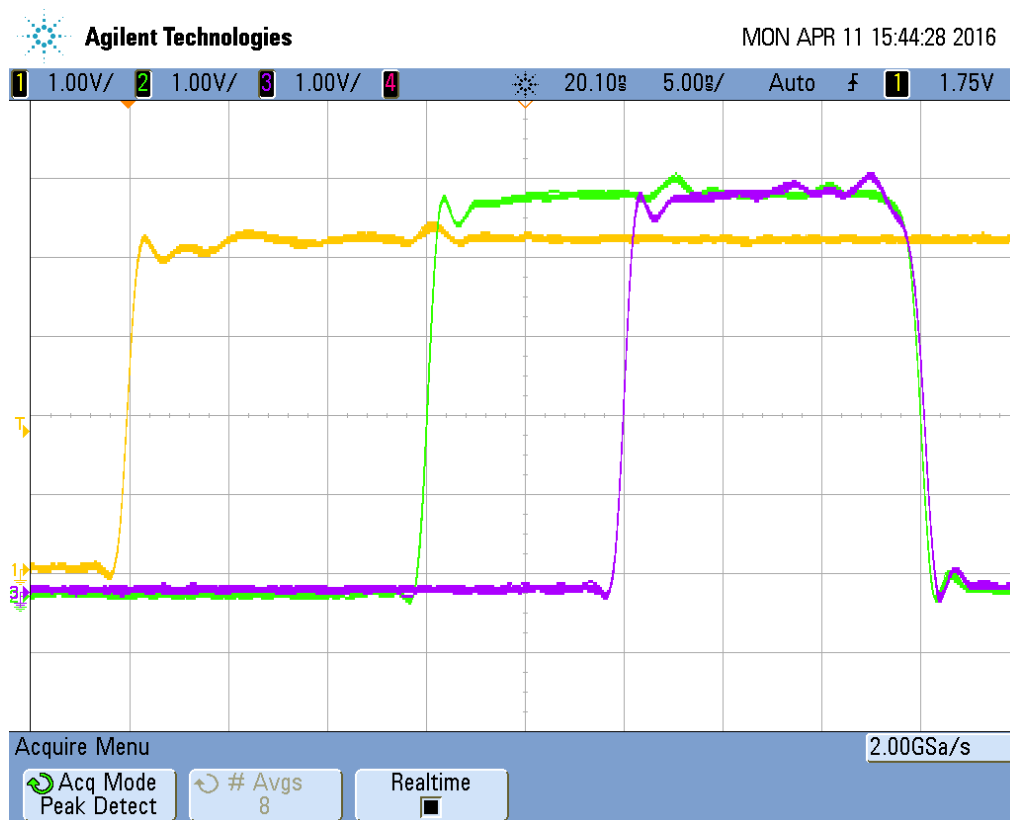
Figure - 16. T1 set to 25ns (in green) and T3 set to 15ns (in purple), T0 reference in yellow
